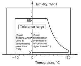
(The allowable temperature range differs for each relay.)
